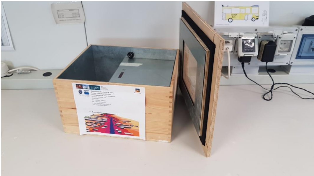
Fig. 1 Reverberation chamber for smartphones calibration; the photo shows the reverberation chamber, with the walls covered by the metal sheet; the lid with a closure seal of expanded rubber with a density of 130 kg/m 3 ; the control window in Plexiglas.
