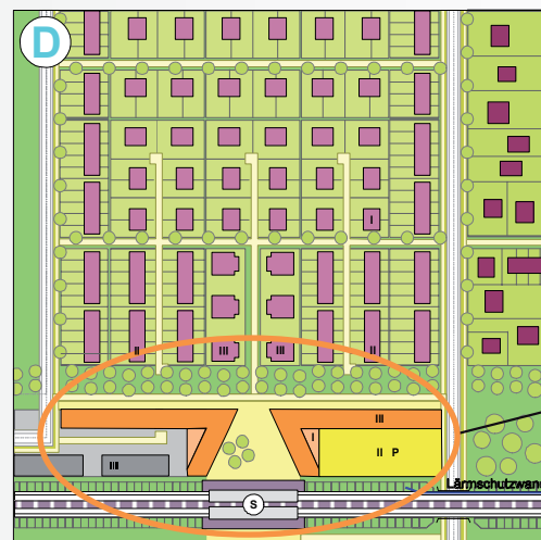
Buildings as noise barriers along a railway line
