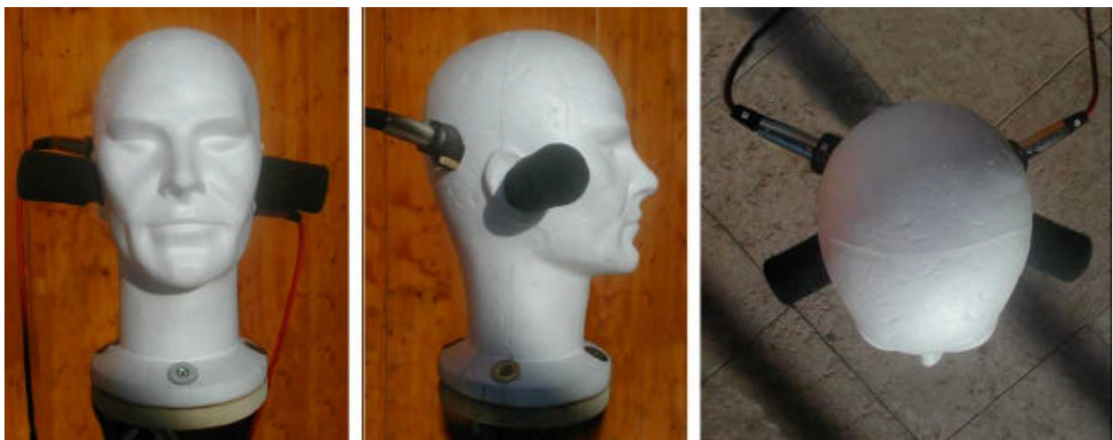
Figure 1. Front, side and top of the binaural dummy head.
