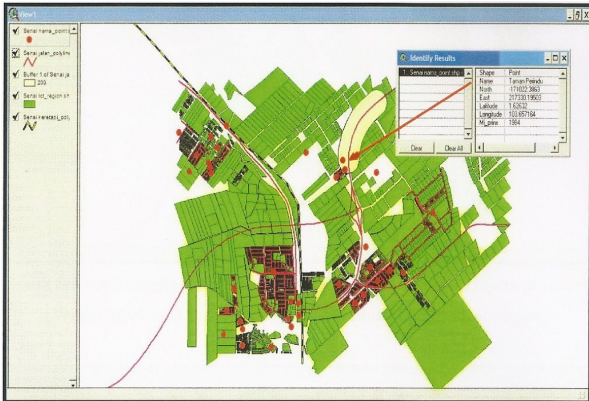
Figure 3: Parcels of residential properties located between 200 meters (inclusive) from noise-emitting trunk road.
